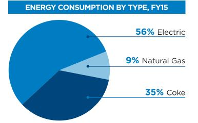
We also track our energy consumption per ton of product shipped so we can capture gains in energy efficiency that may occur even as our overall energy increases due to higher production rates. Our consolidated energy intensity was 10.28 mmBtu/ton of product shipped for 2015.
